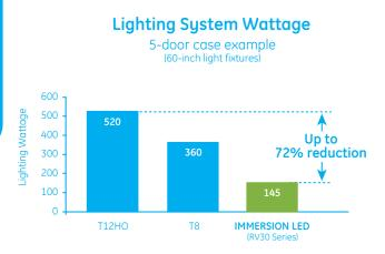
Additionally, for every watt of light reduced inside the refrigerated case, the compressor doesn't need to work as hard to remove the heat from inside.
